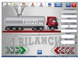
"Weightdosage" is a software which guides the operator during dosing operations. It enables the manqagement of weighings directly from PC, connecting it to the weight indicator, for the dosage in charge.
