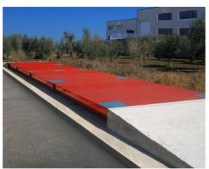
New generation varnished modular weighbridge in floor-level and over-floor variant. It is suitable for weighing trucks, articulated lorries and tractortrailers in the industrial, agricultural and commercial fields. The loading platform is made from embossed steel plates (checkered plates) of big thickness. Functioning with load cells IP68. CE-M approvable.
