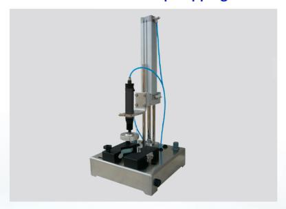
The semi-automatic bench top capping machine, complete with an interchangeable capping head, is suitable for plastic pre-threaded caps, twist-off caps and pressure caps, made entirely of stainless steel. By pressing the two side buttons at the same time, the clamps tighten so that the jar remains stationary, and the head goes down, screwing the cap.
