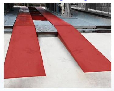
Double lane modular weighbridge varnished or hot-dipped galvanized, in ground level or above ground variant. It is suitable for weighing trucks, articulated lorries and tractor-trailers in the industrial, agricultural and commercial fields. The loading platform is made from embossed steel plates (checkered plates) of big thickness. Functioning with load cells IP68. CE-M approvable.
